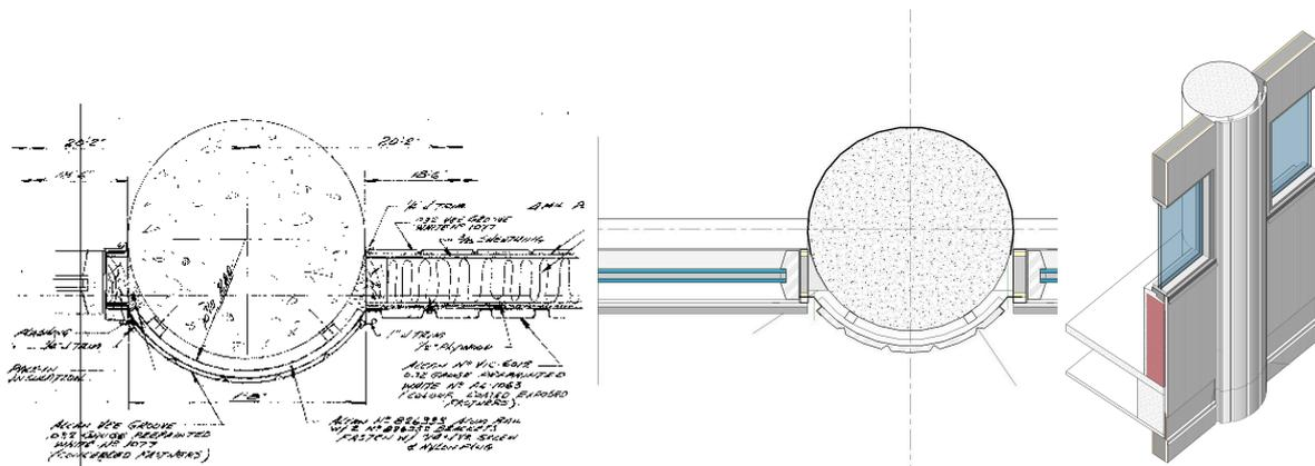
**Figure 4:** (Left to right) Original shop drawings (plan) for 1978 iteration of the factory re-cladding and Revit reconstruction (plan and axonometric).
