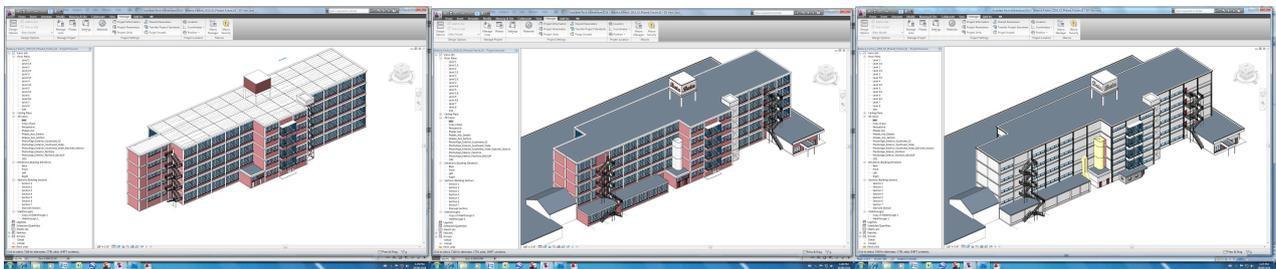
**Figure 5:** (Left to right) Temporal sequence of factory in BIM software, showing the original construction and the subsequent renovation phases.
