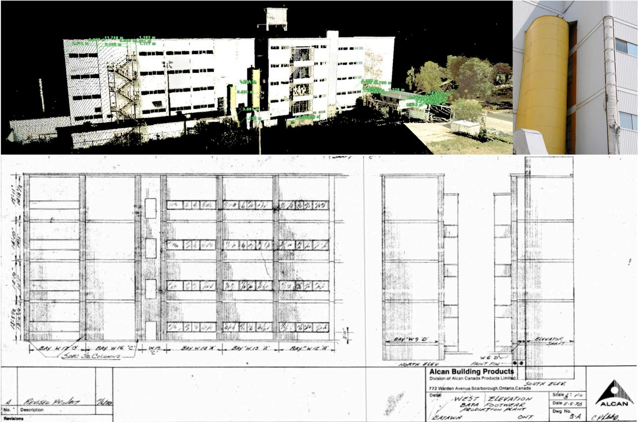
**Figure 3:** Heterogeneous source documents used to construct the factory Revit model, including TLS data, photographs, and construction drawings .
